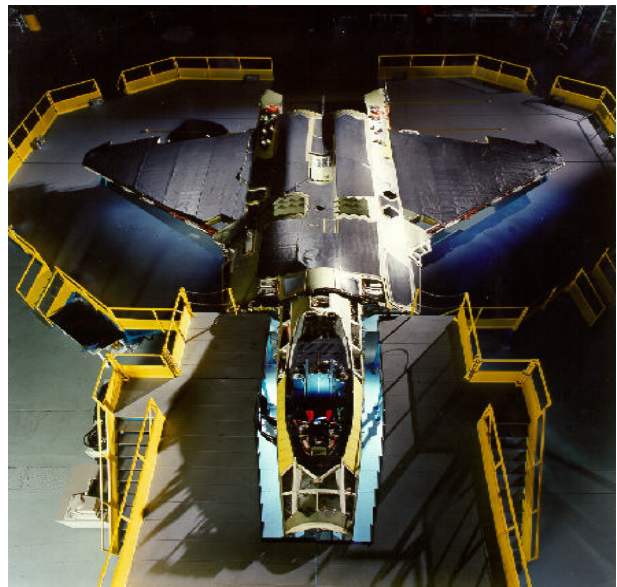
Figure 9: F-22 Assembly Station
